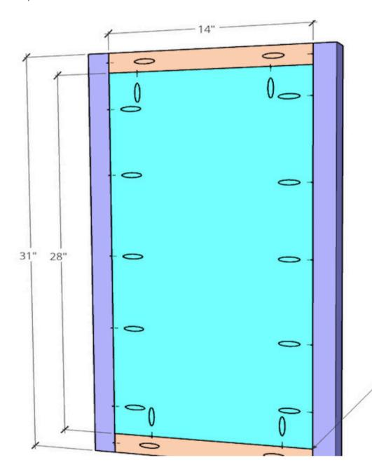
Assemble 2 side panels using 1 1/2" pocket holes with 2 1/2" pocket hole screws on the 2x2s, and 3/4" pocket holes with 1 1/4" pocket hole screws with the plywood panel
