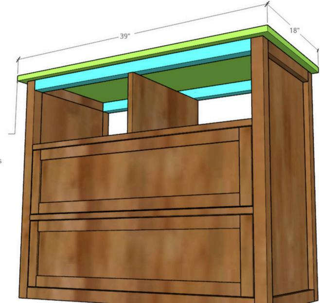
Cut top from 3/4" plywood and place on top of dresser leaving 1" overhang on sides and front. Use 2" wood screws through top 2x2s to attach.
