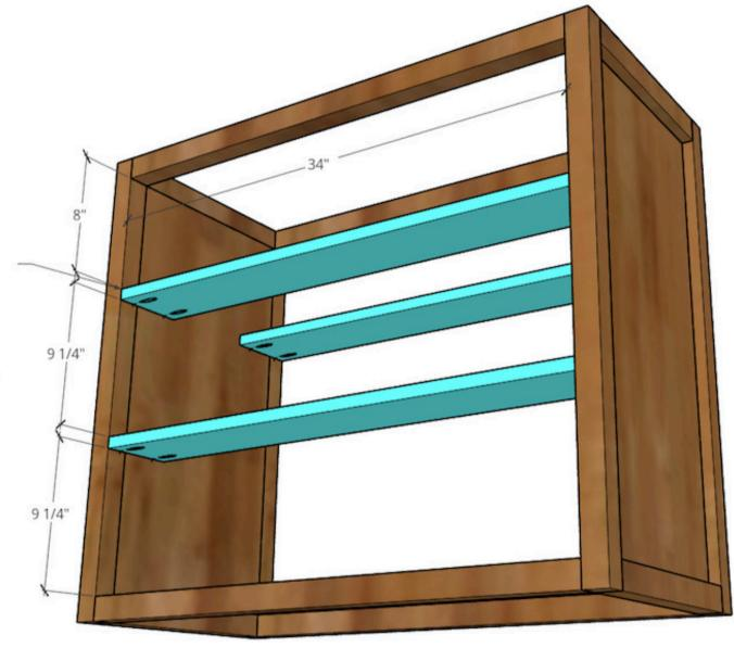
Install 3/4" plywood drawer dividers using 3/4" pocket holes and 1 1/4" pocket hole screws. Two at top (front and back) and one at bottom in the front.
